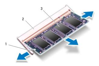
1 securing clips (2) 2 memory-module connector
